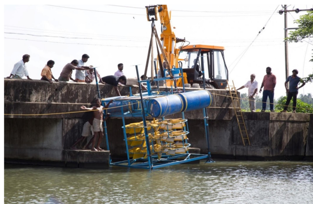
Vertical axis water wheel which generates electrical energy from tidal wav
